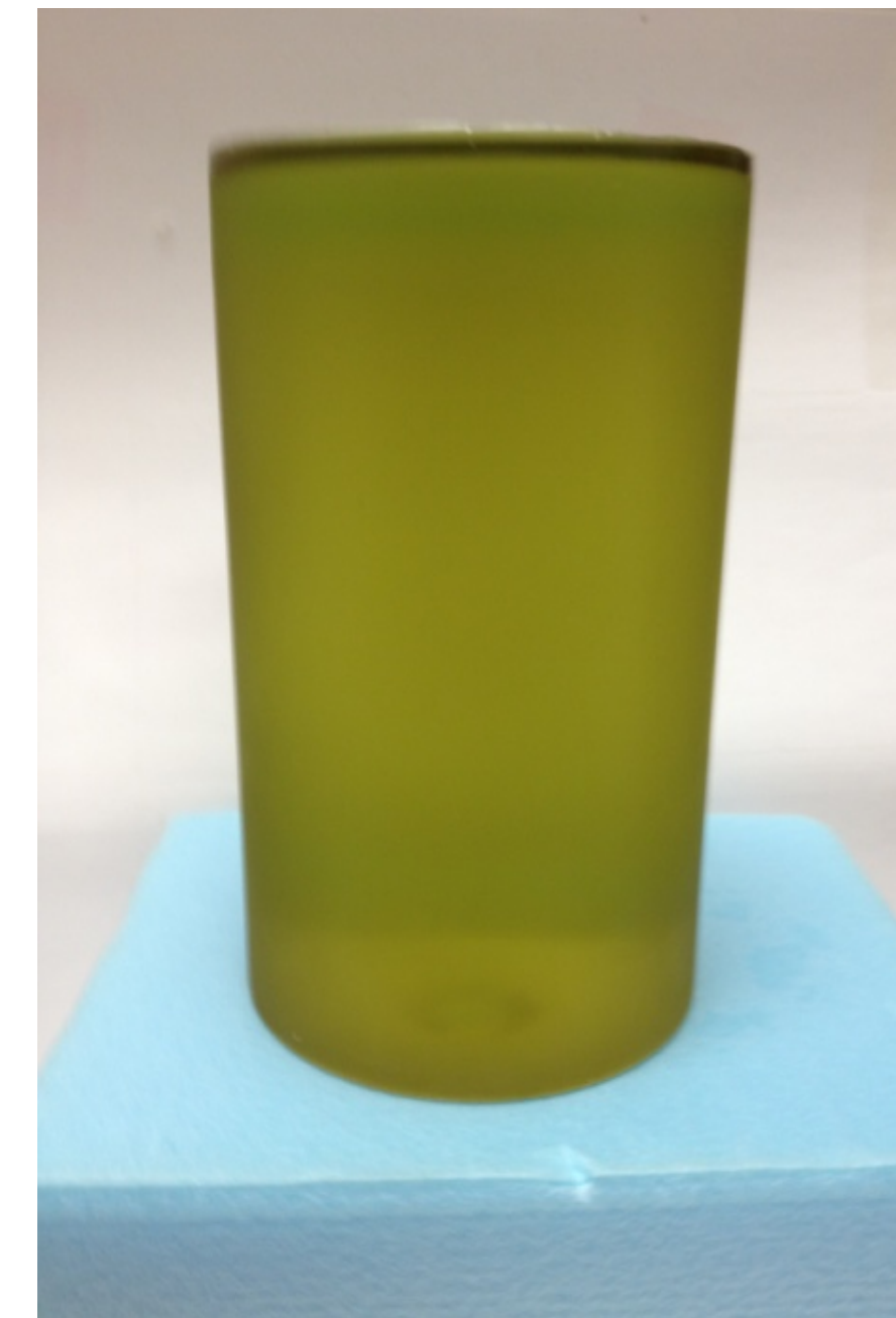
Figure 3 (right): A PRESAGE® dosimeter formulated for high-LET dosimetry.
