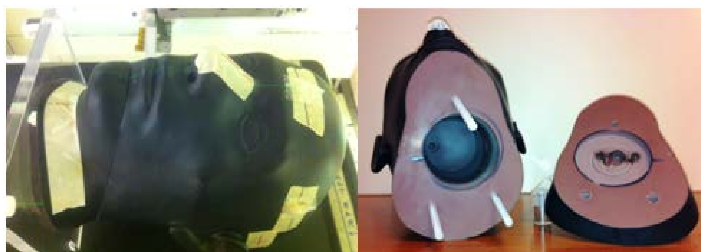
Figure 1: The RPC anthropomorphic head phantom used in proton irradiations.
